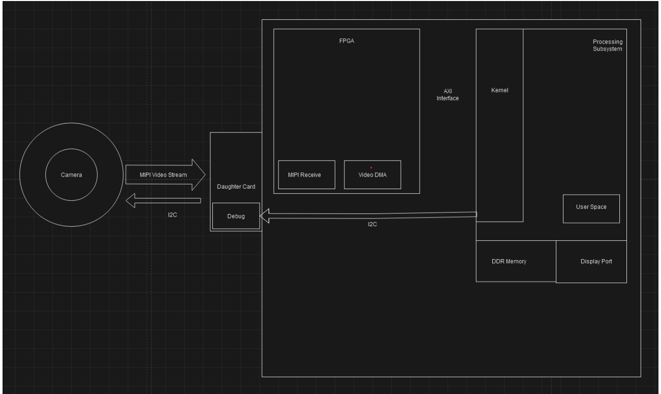
Block diagram for the video pipeline for machine learning computer vision.
